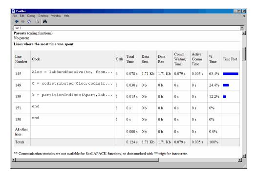
The code that is displayed in the report is taken from the client. If the code has changed on the client since the communicating job ran on the workers, or if the workers are running a different version of the functions, the display might not accurately reflect what actually executed.
