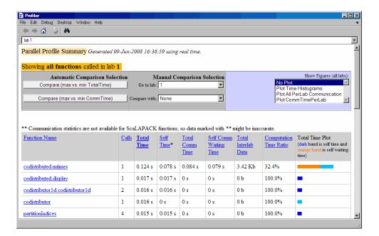
The function summary report displays the data for each function executed on a worker in sortable columns with the following headers:
